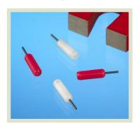
The inputs for these nonmagnetic PinPorts and portto-tubing connectors are made with Nitinol tubing instead of stainless steel. The injectors included with the ports do still include stainless steel tubing as it is assumed these will be used for intermittent access outside the magnetic field.
