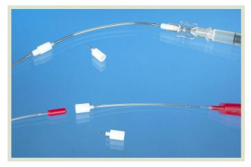
Use a PinPort connector to access a PinPort at the end of a segment of tubing. Applications include acute experiments where tethering is not necessary, or external tubing connections where the self-sealing septum in the PinPort is helpful.
